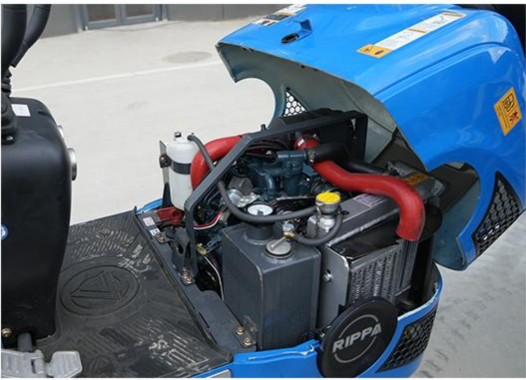
3 Fully openable bonnet Completely destructible, it is convenient to change the fuel system and the fuel system in daily life.
