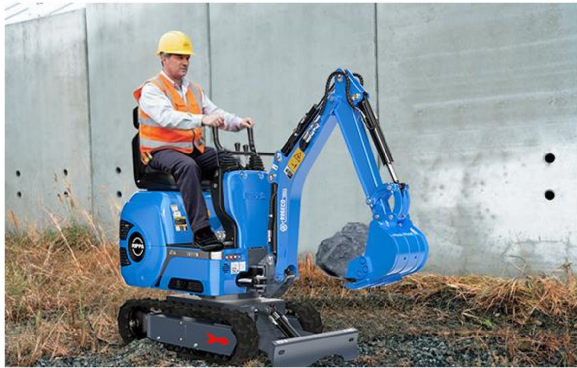
9 Rear boom cylinder You can work without worrying about damaging the boom cylinder when scooping large stones or concrete pieces with the bucket, loading them into a dump truck, or using an on-board breaker.
