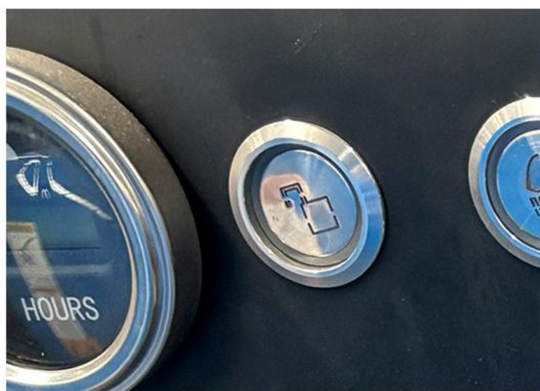
2 Operation lock button Machine operation is only permitted when the operating lock is open, enhancing machine safety and preventing accidental operation.
