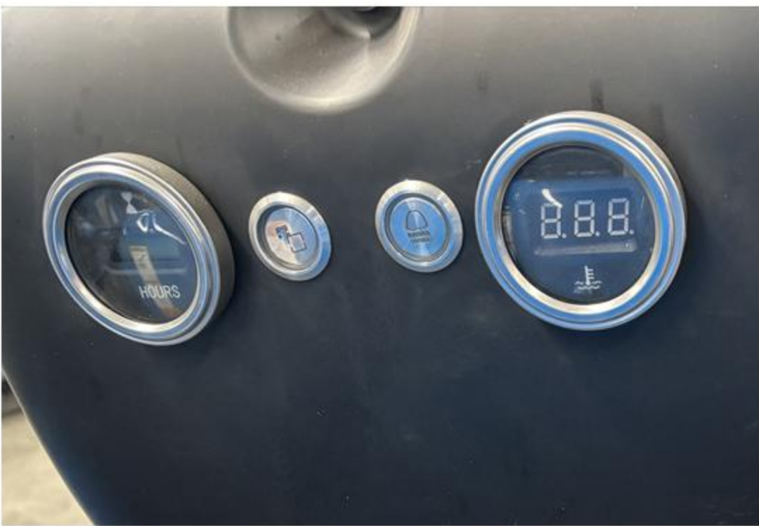
7 Display Instrument It can display the machine's operating time and parameters such as machine temperature.
