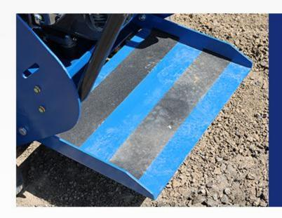
The footrest can be flippedup and is equipped with a pinfor connecting and hingedparts. It can be fixed androtated flexibly, which is con-venient for disassembly, as-sembly and maintenance.
