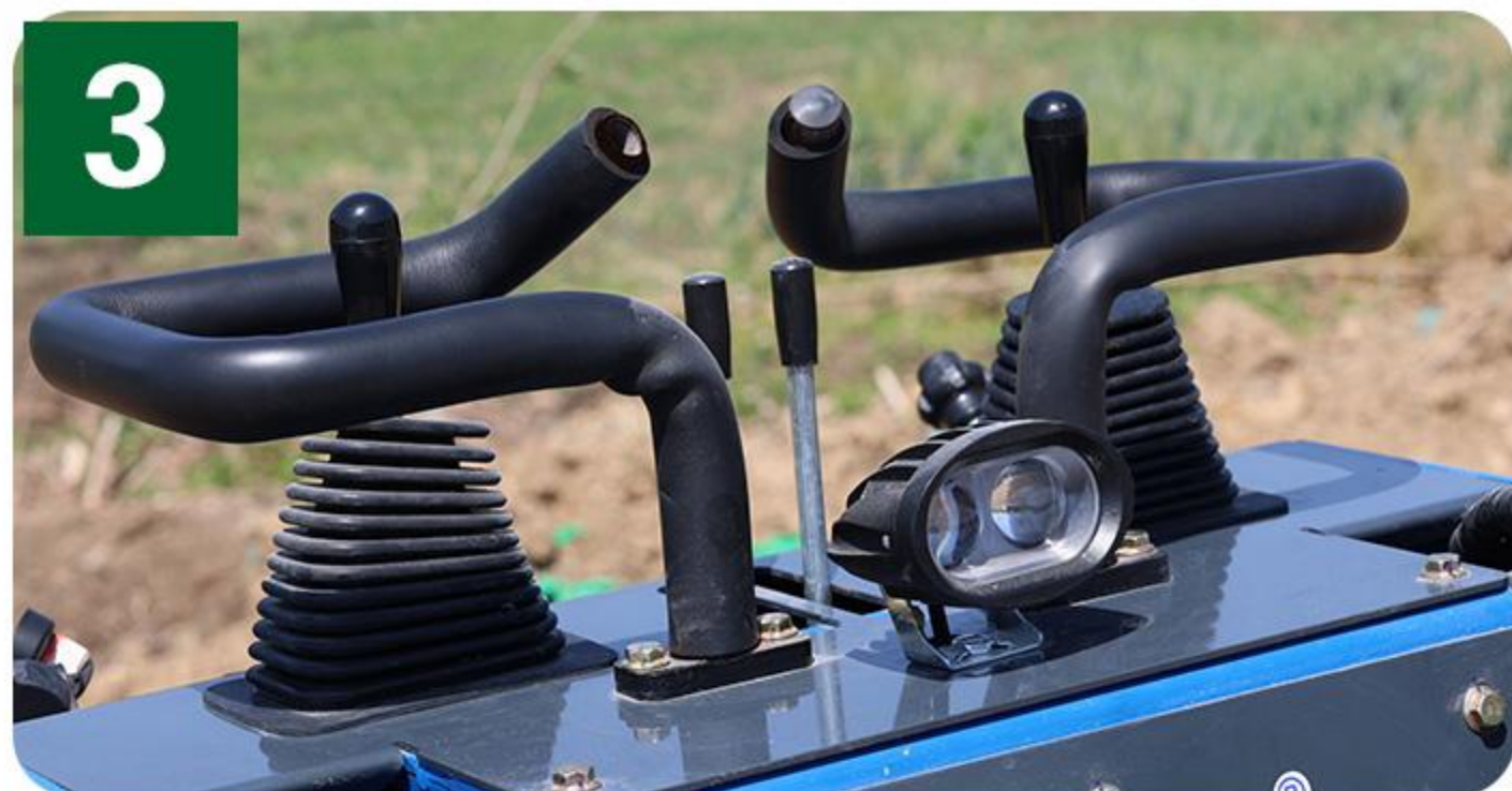
Operating handle A single lever realizes forward, backward, steering and other actions, which is convenient for operation and has high and low speed functions.
