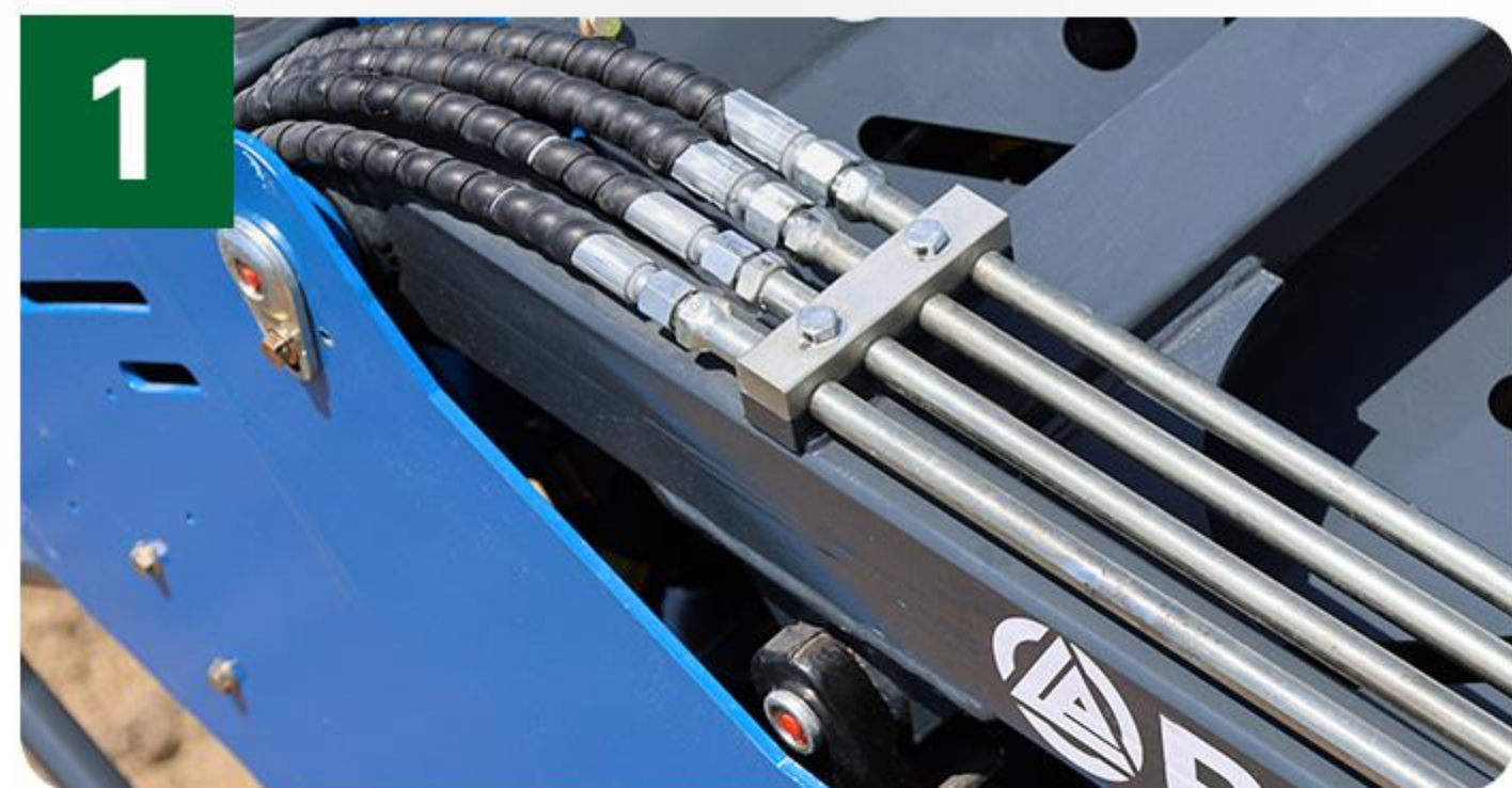
Oil pipeline A metal oil pipe is used above the robotic arm, which is not easily damaged during work.
