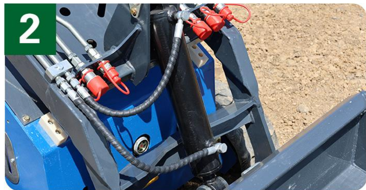
Oil cylinder Inverting the cylinder can effectively protect the cylinder rod from damage and extend the service life of the cylinder.
