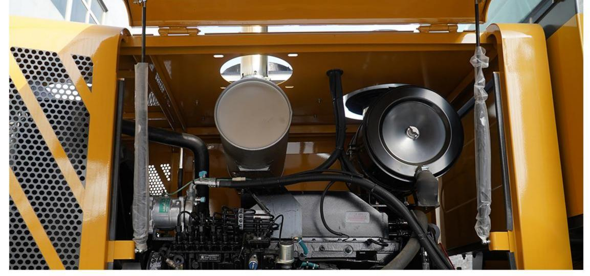
The large-opening hood can be opened upward 90°, providing a large space for maintenance; the air filter and fuel filter are centrally arranged.
