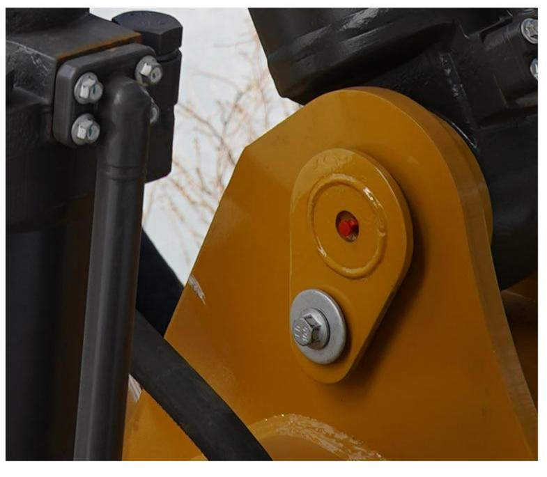
External lubrication points: The grease lubricating oil pipes are drawn out from the pin shaft and bushing, making maintenance easy.
