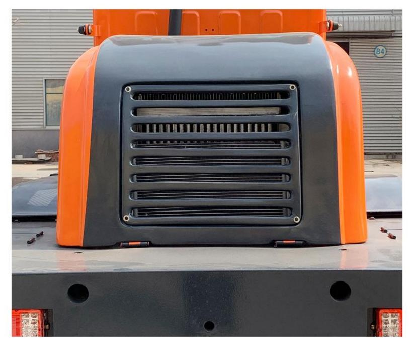
The horizontal radiator has small medium flow resistance and good heat dissipation effect.
