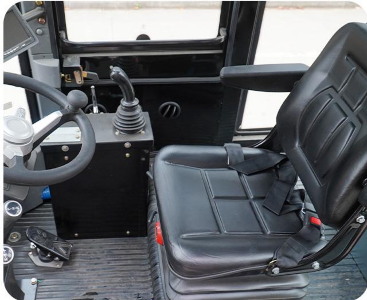
Comfortable safety seat equipped with shock absorption function to provide a more comfortable use
