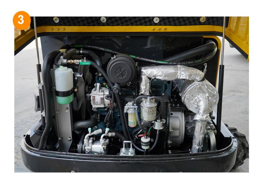
The R350 3.5-ton mini excavator can be equipped with Kubota engine/Changchai engine/Xinchai engine to meet the needs of different countries at home and abroad;
