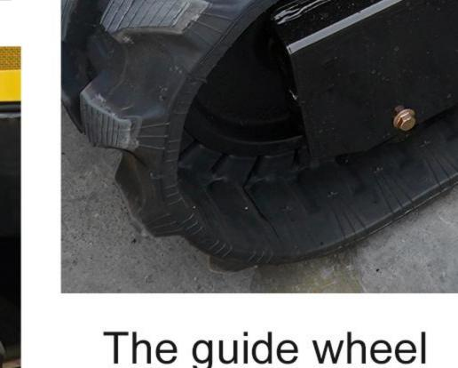
The guide wheel and tensioner can guide the direction and tighten the track.
