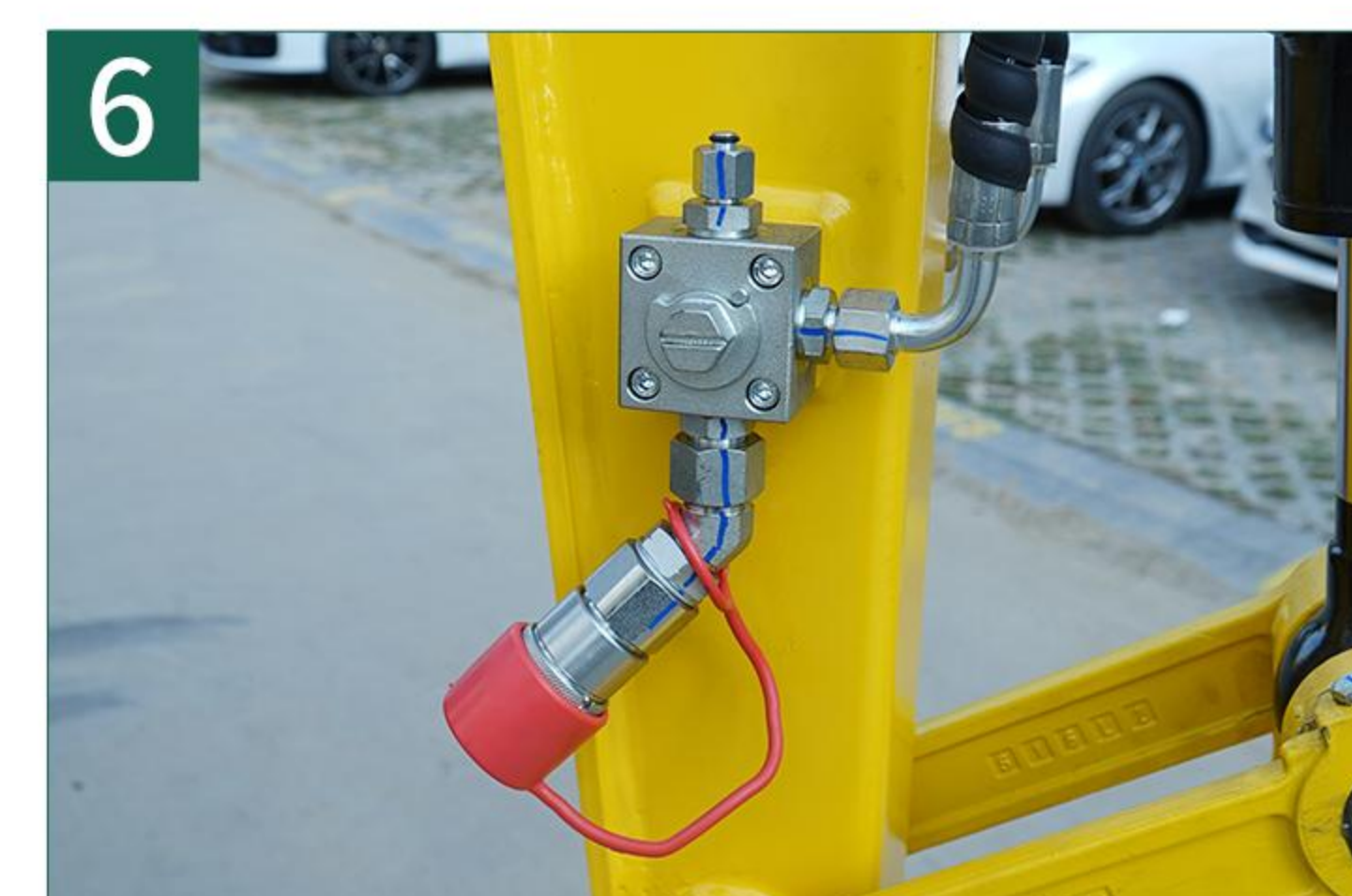
Crushing hammer shut-off valve
